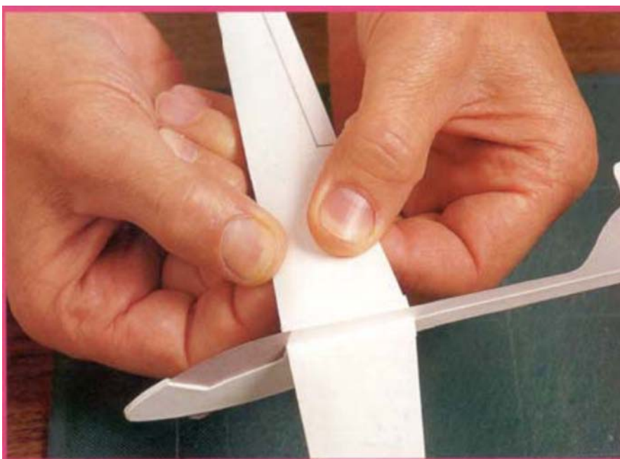
Figure 11-7-5 Adjusting Wing Curvature (Camber)
