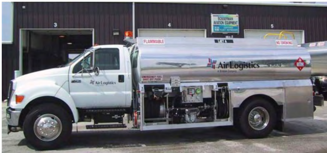
Figure 16E-13 Refuelling Cabinet
