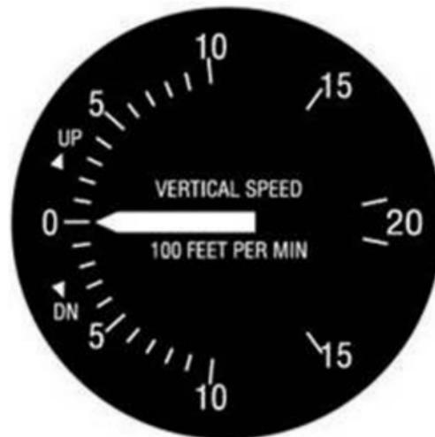
Figure A-4 Vertical Speed Indicator
