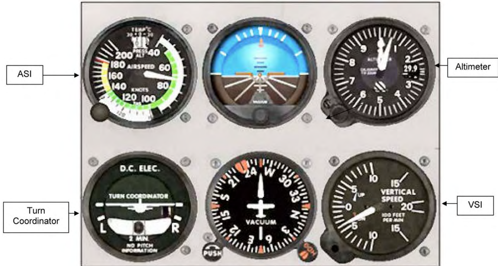
Figure A-1 Cessna Flight Instrument Panel
