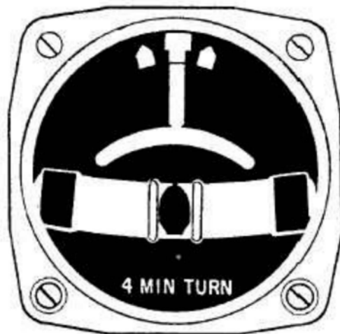
Figure A-8 Turn and Bank Indicator
