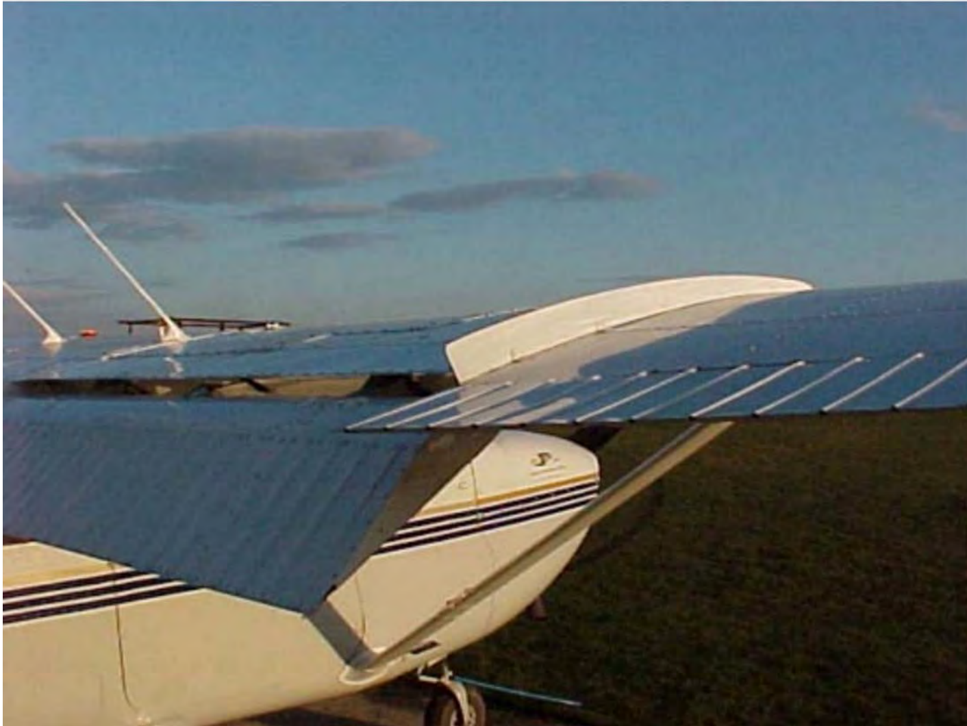
Figure A-9 Wing Fences
