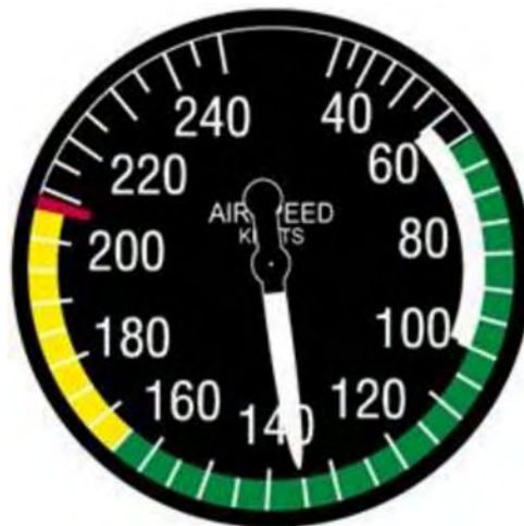
Figure A-2 Airspeed Indicator
