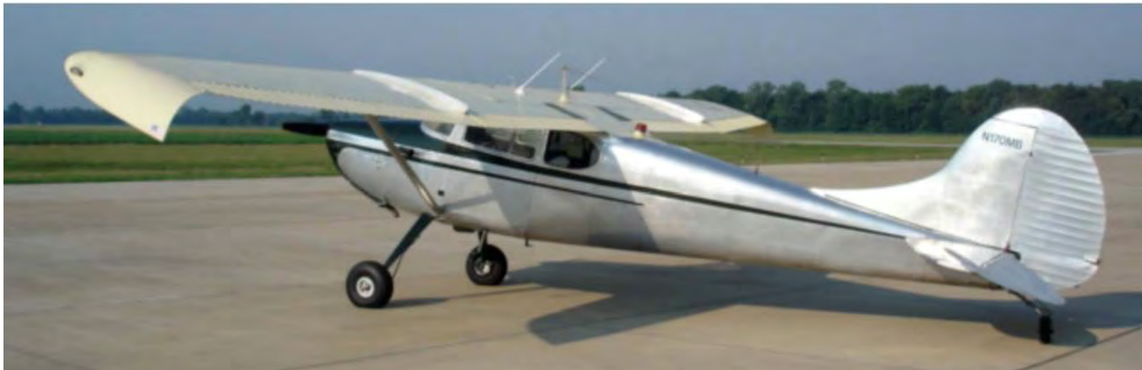
Figure A-8 Drooping the Wing Tips
