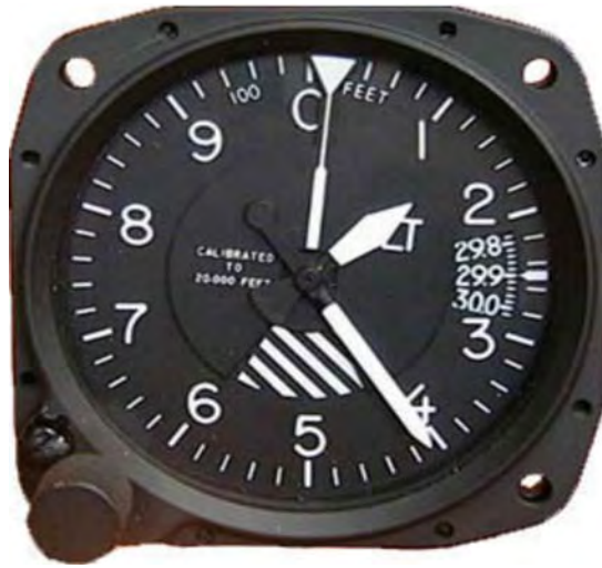
Figure A-3 Altimeter
