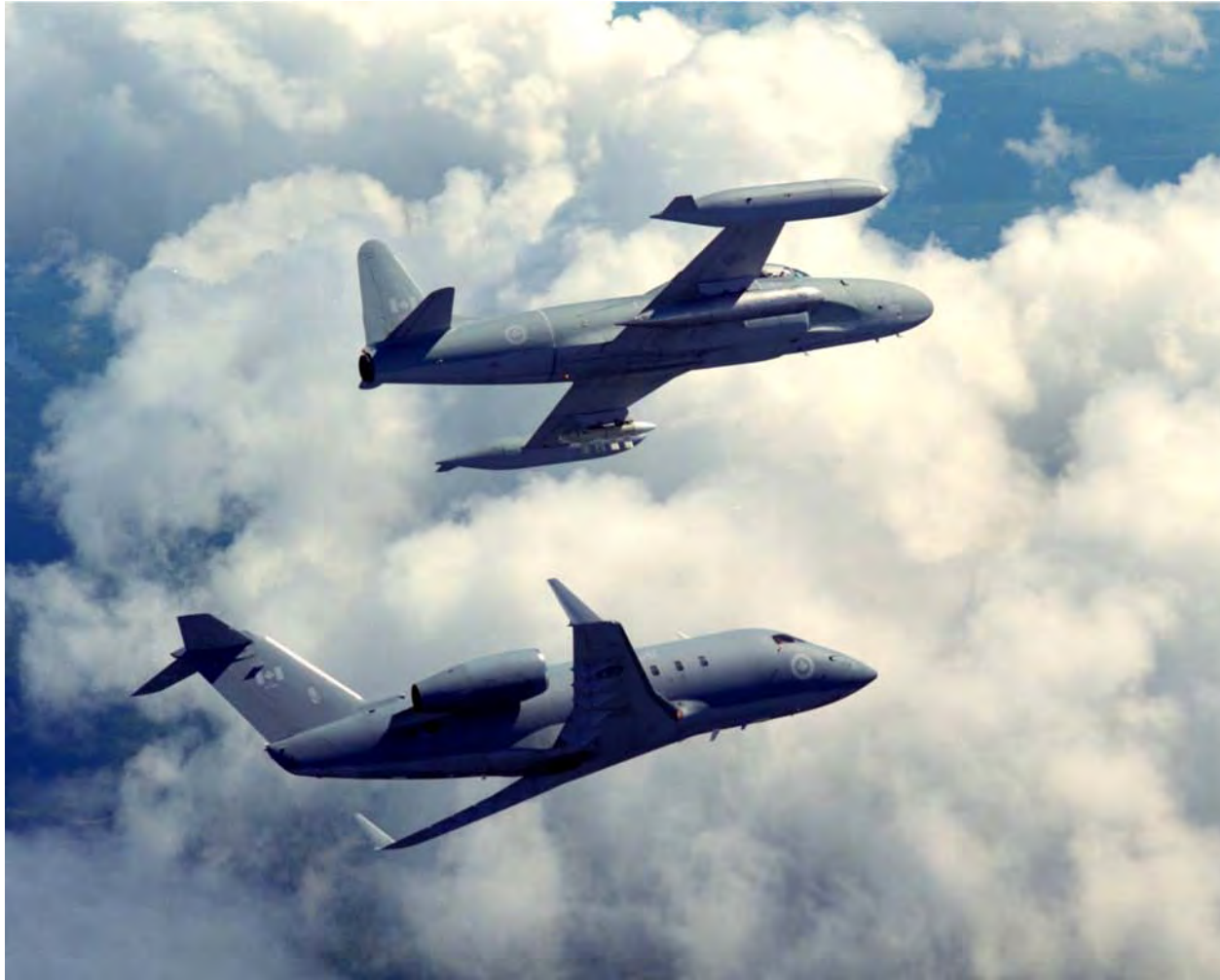
Figure A-7 Wing Tip Tanks and Winglets
