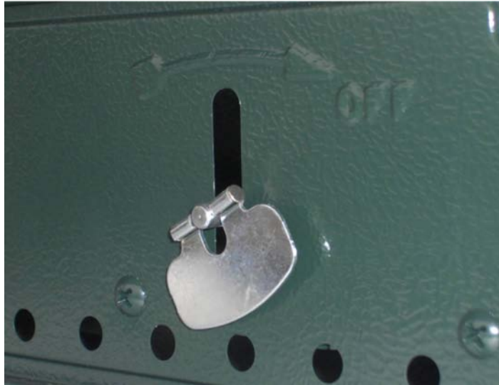
Figure 8 Auxiliary Burner Control
