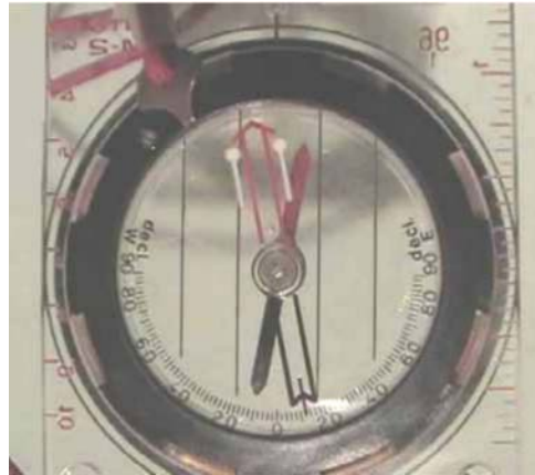
Figure 5 Declination Scale and Screw
